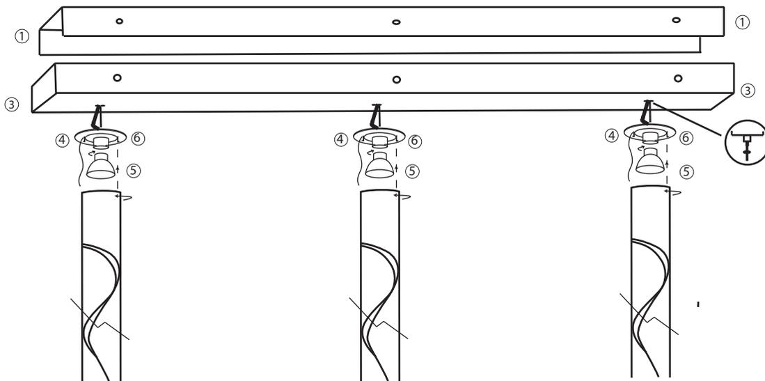
SPARE SOME CENTIMETRES OF THE WIRE BEFORE CUTTING THE REMAINING PART.
